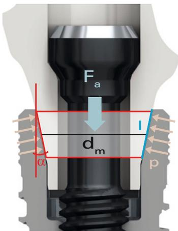
Joint compression ( $p$ ) depends on a number of variables such as preload (tensile force  $F_a$ ), friction angle ( $\alpha$ ) and contact length ( $l$ ). Small changes in any of these parameters can lead to extreme load and stress conditions, which can cause implants to fracture.
