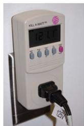
**3 Use a Kill A Watt™ meter:** RPU has a number of Kill A Watt meters that you can use in your home for free! This device will tell you how much electricity products are using
