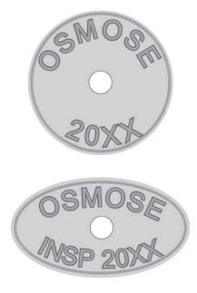
This round tag represents an inspection via a full 18" excavation and treatment with an approved paste. The tag shows CONTRACTOR's name and the actual year the work is performed.
