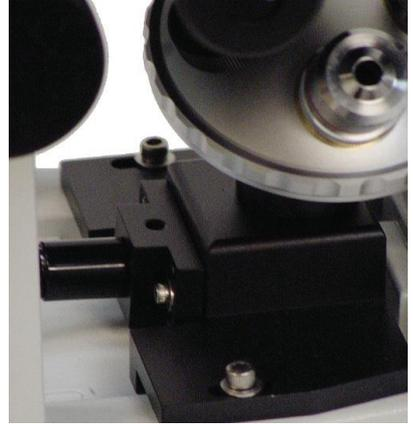
1. Using a 3/32" hex wrench, loosen the two screws on either side of the light source mount.
