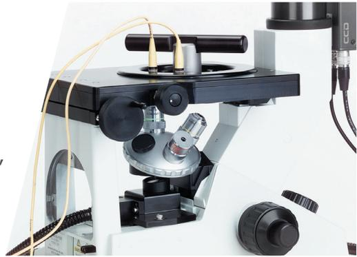
The ME-12013 LED/ME-12015 Controller operates from a 24 volt DC output power adapter (ME12015) with switching transformer to accept AC voltage 90-240 volt, 50-60Hz for domestic or international use. This unit is used to power both the CCD camera and the illumination of the microscope.
