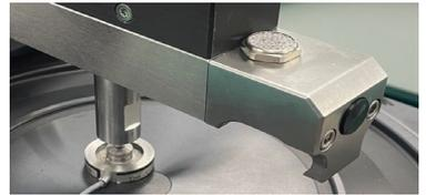
4. Allow external master load cell 15 minute of warm up before starting calibration.
