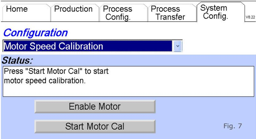
After selecting "Enable Motor", select the "Start Motor Calibration" button. This will activate the Platen to rotate at different speeds and calibrate the internal electronics. Once it is complete select the "Accept" button to save calibration.
