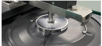
4. Plug the USB connector of the EZ-CAL Load Cell into the side USB port of the polishing machine.
