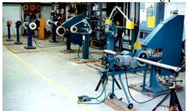
time, hindsight was getting better, and we knew we couldn't automate the project or handle it in a conventional manner. It was proposed and I agreed that the job could possibly be accomplished using swing frame polishers and buffers. These are counter balanced abrasive belt heads and buff heads which are suspended from above and operated by manpower from the floor. The units were
