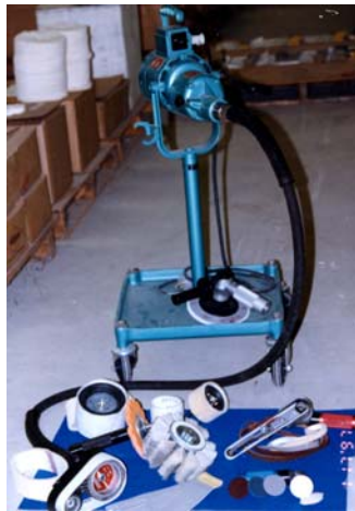
Figure 4: A three-phase, 7 speed flex-shaft system.
