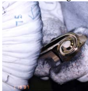
Figure 11: The third step of the finishing process for castings uses a 14 inch white untreated buff with Y86 mint green compound.
