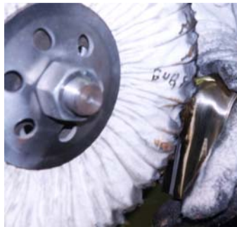
Figure 10: A 14 inch white dip treated buff with X67 Tripoli compound is used for the second step of finishing the castings.
