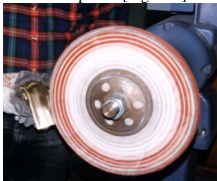
Figure 8: Finishing the castings (step 1).
