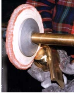
Figure 9: A 6 inch spiral sewn buff with 180 grit greaseless compound.
