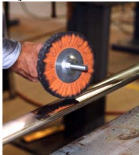
Figure 1: A 6 inch orange mill treat buff is used with X67 Tripoli (brown) cut compound.
