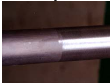
Figure 8: The left side of this 2 inch tubing is raw, while the right features a #3 finish.
