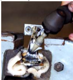
Figure 6: Hard-to-reach areas can be accessed with a portable die grinder using an alligator mandrel.
