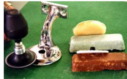
Figure 7: Final touches are applied with a portable die grinder and mechanical locking CLEO® buffing discs.
