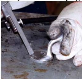
Figure 5: A portable tool with structured abrasive belt.
