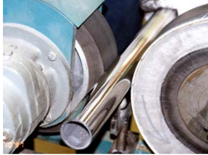
Figure 9: An abrasive centerless machine brings this aluminum tubing to a #7 - #8 mirror finish.
