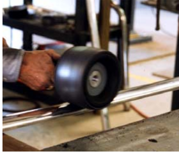
Figure 2: Shown is a 5 inch inflatable wheel with a CLEO Buff-Belt with X67 Tripoli (brown) cut compound.
