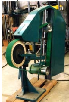
Figure 10: A 2 h.p. "space saver" abrasive belt machine.
