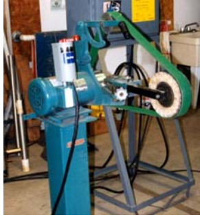
Figure 3: A pedestal mounted BM2 abrasive belt machine.
