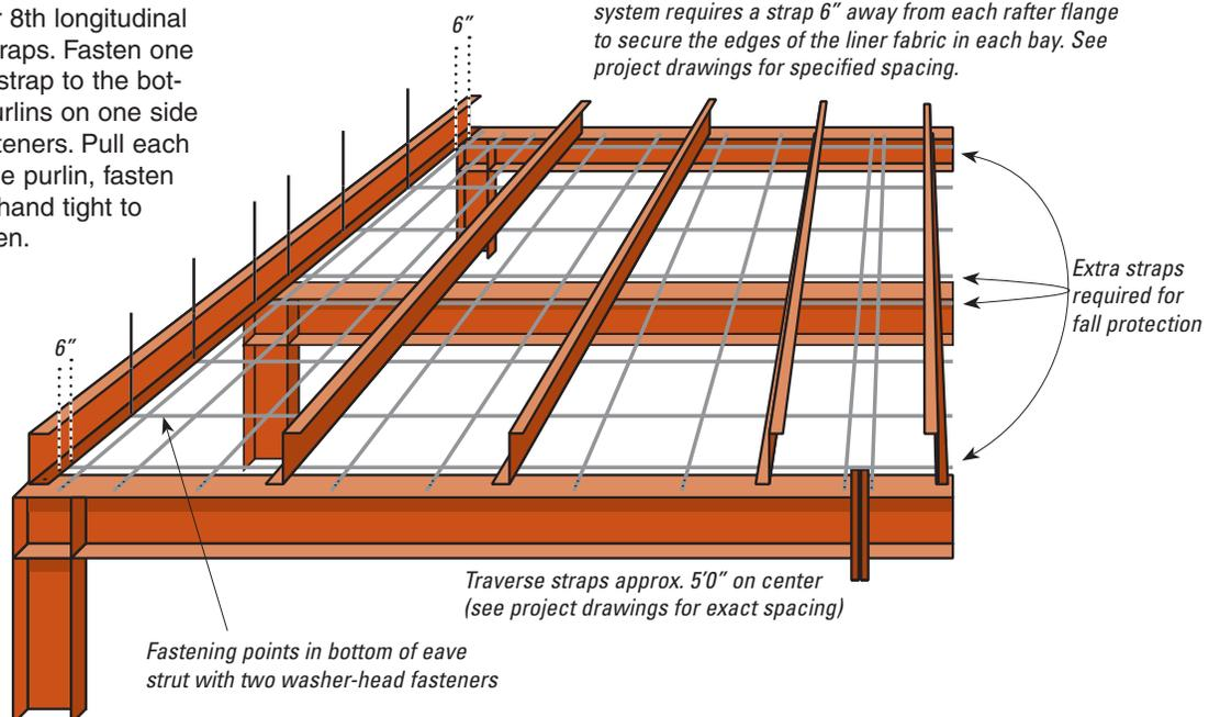
**Step 3:** Place the liner fabric on the steel strap platform in the eave purlin space and clamp two corners of the fabric. Feed the other end of the fabric underneath the purlins and pull tightly over the platform of straps to the ridge. Fasten the fabric and straps to the bottom of the nearest ridge purlin then continue to pull the fabric to the opposite eave purlin. Fasten all straps at purlin intersections.
