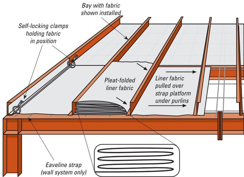
**Step 4:** Trim the edges of the fabric to fit around the points where the purlins are fastened to the rafters and seal the fabric to the top of the rafters with contact sealant.
