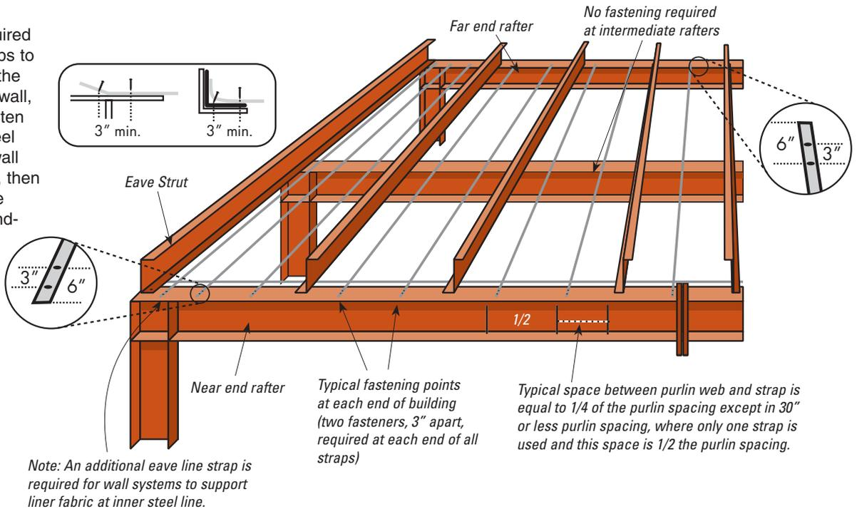
**Step 2:** Pull traverse straps across building width, over every 6th or 8th longitudinal strap, and over the ridge straps. Fasten one end of each traverse steel strap to the bottom of the sidewall eave purlins on one side of the building with two fasteners. Pull each strap hand tight to one ridge purlin, fasten strap, then pull each strap hand tight to the opposite eave and fasten.
